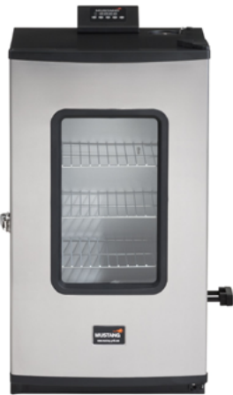
Mustang ELECTRIC SMOKER ELECTRONIC The easy-to-use mains-operated electric assistant gives fish, meat and vegetables a tasty smoke aroma. Power 650 W, 230V-50Hz. 4 gratings, 37 x 33 cm. Brushed steel door with window glass. Digital control panel on top of the smoker. Temperature menu 38-137 degrees. Timing 0 - 24 h. The grease tray also acts as a liquid tray. Smoking chip tray on top of the heating element. The pull-out filling cylinder allows smoking chips to be added to the smoker during smoking without the need to open the smoker door. Includes PVC cover. Warranty 1 year.
